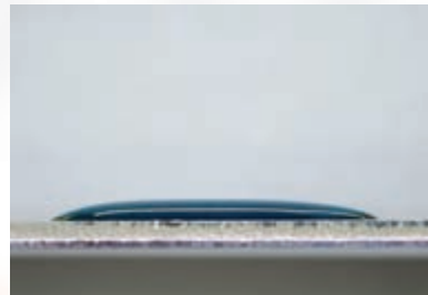
Water drop on plasma treated metal
